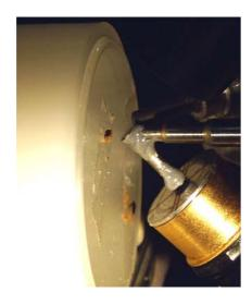
Figure 1. Sample holder (left) supporting a small piece of varnished wood originally of a violin made by G.B. Ceruti around 1800 is presented to the proton beam (right).
