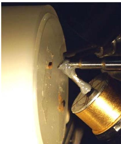
Figure 1. Sample holder (left) supporting a small piece of varnished wood originally of a violin made by G.B. Ceruti around 1800 is presented to the proton beam (right).
