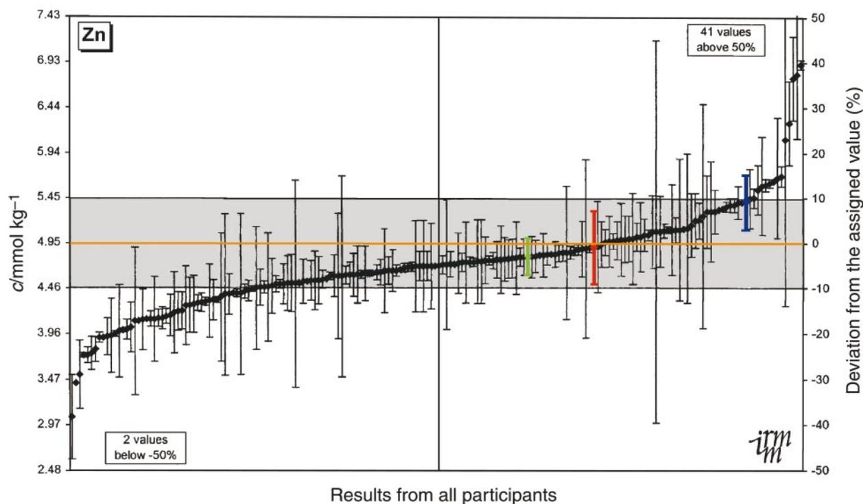
**Fig. 3** Results from all participants of IMEP-14, related to the content of Zn in the sediment sample.<sup>1</sup> The shaded band gives the reference value and the uncertainty interval. Green: FAAS, blue: ICP-MS and red: TXRF at ISAS, Dortmund.
