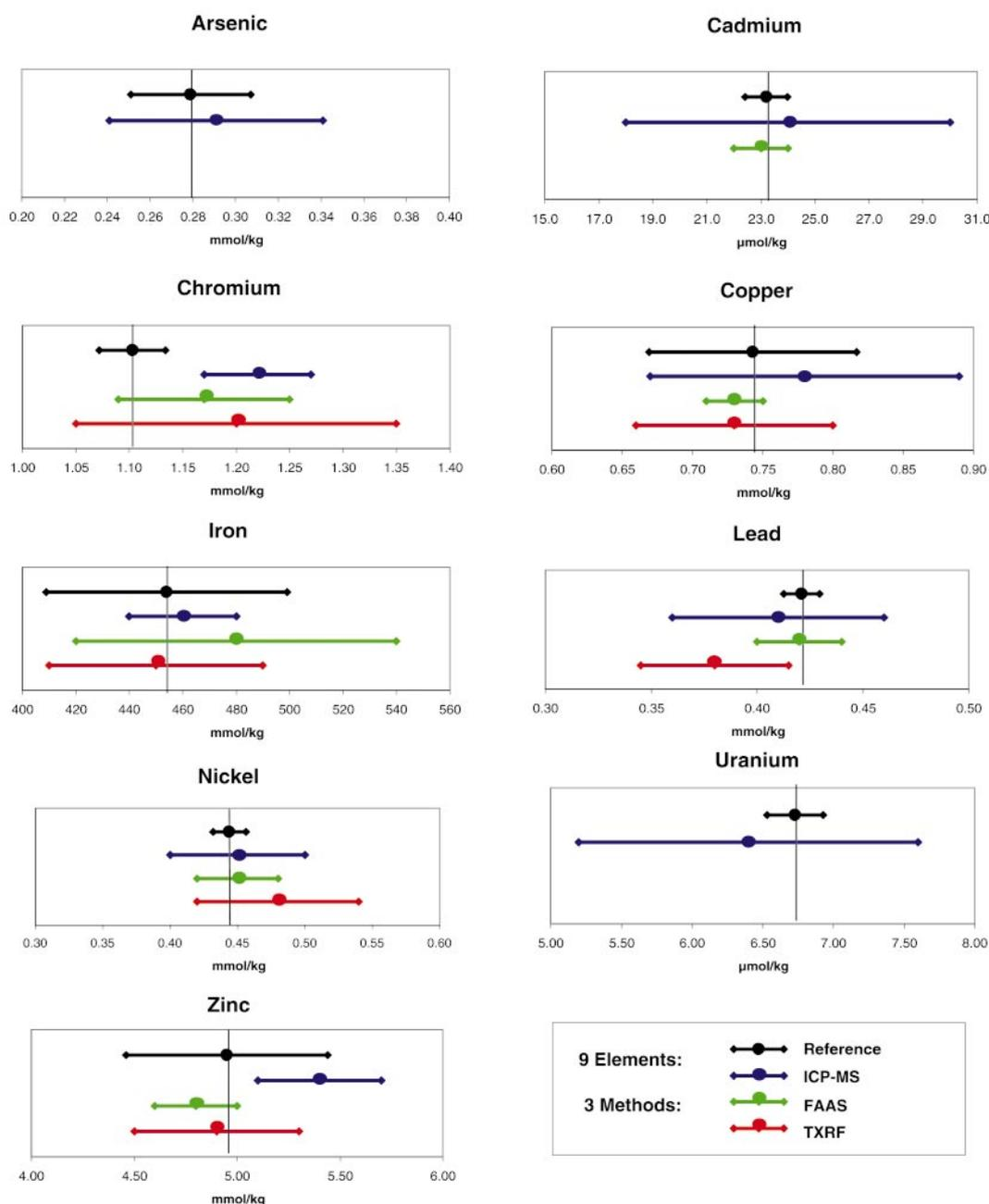
**Fig. 1** Results found for the different elements in the sediment sample with mean value and uncertainty interval. Green: FAAS, blue: ICP-MS, red: TXRF; black: reference.<sup>1</sup>
