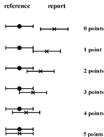
**Fig. 2** Different overlappings of the uncertainty intervals of reported and reference values. The degree of overlapping was expressed by a figure of merit (between 0 and 5 points).
